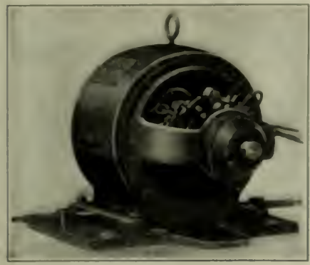
FIG. 292. WESTINGHOUSE MULTIPOLAR GENERATOR
